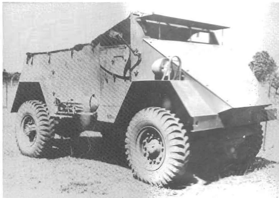
The 4 x 4 vehicle with canvas canopy erected. Note that this has full mudguards on the front. The driver's visor is open and the driver's door flap is down.
