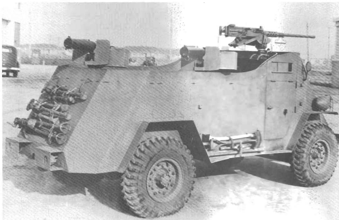
The prototype viewed from the right side. The stowage of the machine gun tripods on the rear hull, and the pioneer tools on the right side can be seen.
