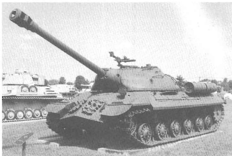
The IS-3 at APG. Note the homemade rear drive sprocket.
