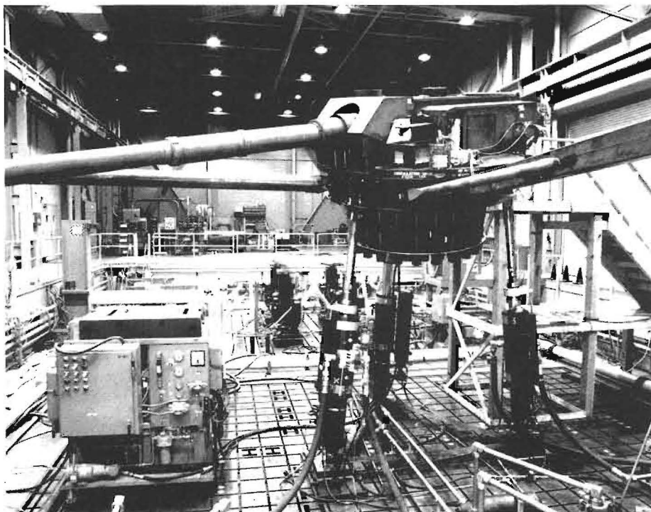
Figure 4. Tank Test Bed Turret on Vehicle Motion Simulator at TACOM.
