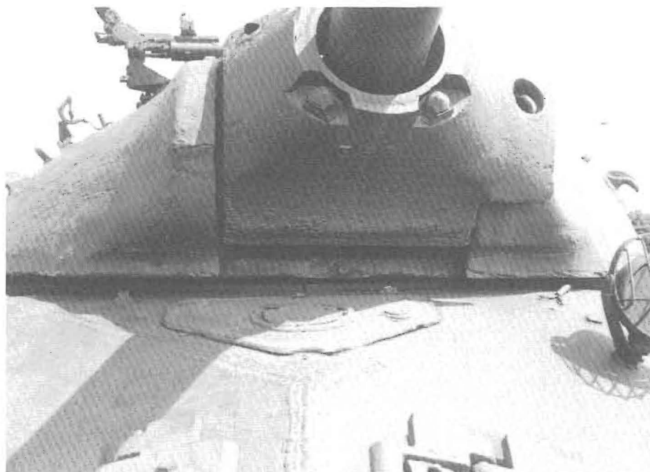
The heavy casting of the turret mantlet and the flat driver's hatch are evident here.
